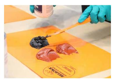
For mixing small quantities of Belzona® 4301 use 2 parts Base to 1 part Solidifier by volume.
