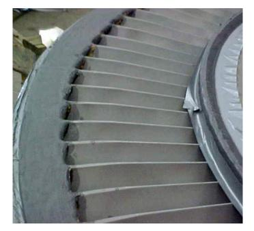
Belzona 1511 (Super HT-Metal) is a high temperature, paste-grade system for rebuilding equipment damaged by erosion-corrosion. This material can also be used as a high-strength structural adhesive or for the creation of irregular load bearing shims.
