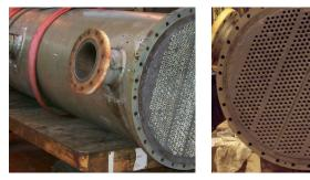
Heat exchanger tube face damaged by severe galvanic and pitting corrosion. Rebuilt with Belzona 1511 prior to the application of a Belzona high temperature coating.
